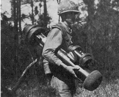
Among the many weapons systems evaluated in 1971 is the shoulder-fired MX47 Dragon anti-tank system. The weapon consists of reusable tracker, rocket-powered missile and disposable launcher.
